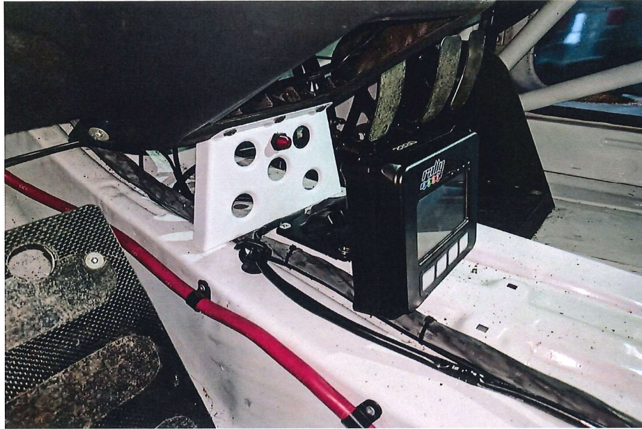
The RallySafe unit then mounts to the 25mm rubber ball mount (connected through the RallySafe connector).
