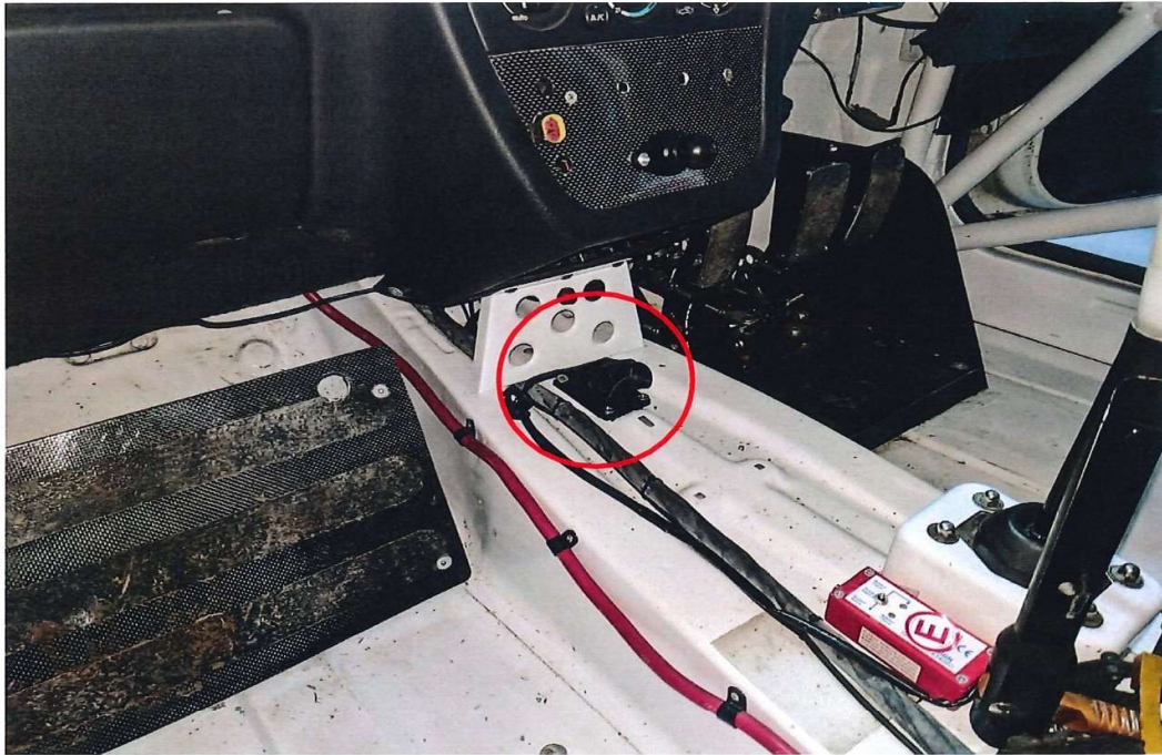
Here the 25mm rubber ball mount is securely attached to the tunnel.
