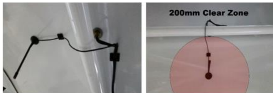
Figure 3. The internal antenna must be at least 200mm away from any roll cage components
