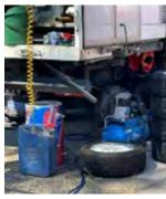
Spill trays under fuel drum and generator are not in place
