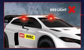
A flashing red light, along with an alarm sound, means the car is unsafe. No light means it is potentially unsafe. Only touch the car if there is a green light.
